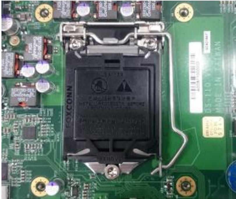
2. Press the CPU socket lever and pull it aside away from the socket to unlock it. Pull back the lever to open the socket.
