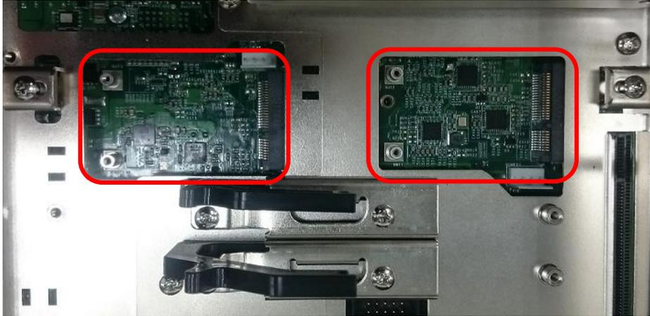
2. Tilt the Mini-PCle module at a 45 degree angle and insert it to the slot until the gold-pated connector of module contacted firmly with the slot.
