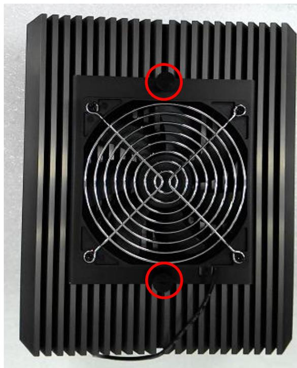
4. Connect the FAN cable to external fan power connector at rear panel.
