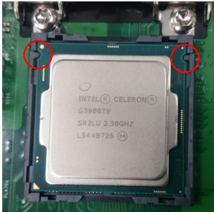
5. Place the thermal pad on the CPU heat spreader. Press down the socket lever to lock the CPU.
