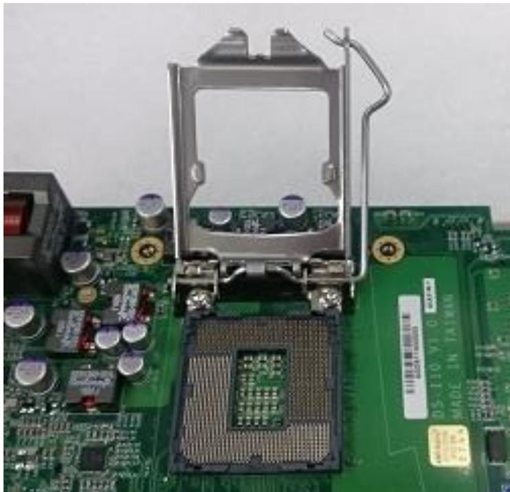
3. Align the notches on CPU with the alignment post on socket.
