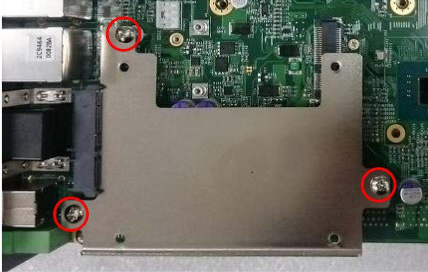
2. Make the PCB side of the HDD face up, place the HDD bracket on it. Ensure the direction of bracket is correct and use 4 provided screws to assemble HDD and HDD bracket together.
