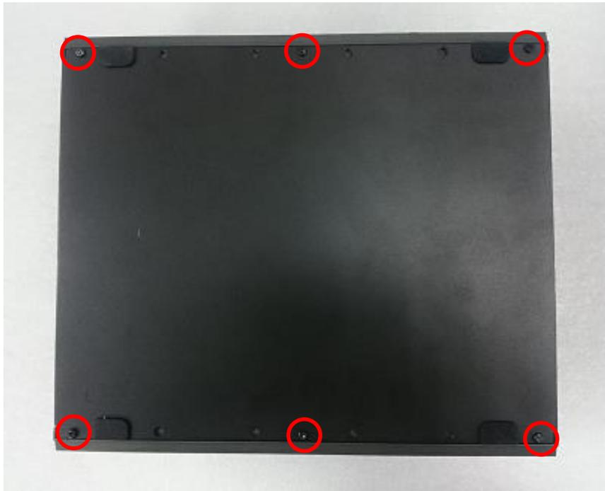
2. Remove the bottom cover from the chassis.
