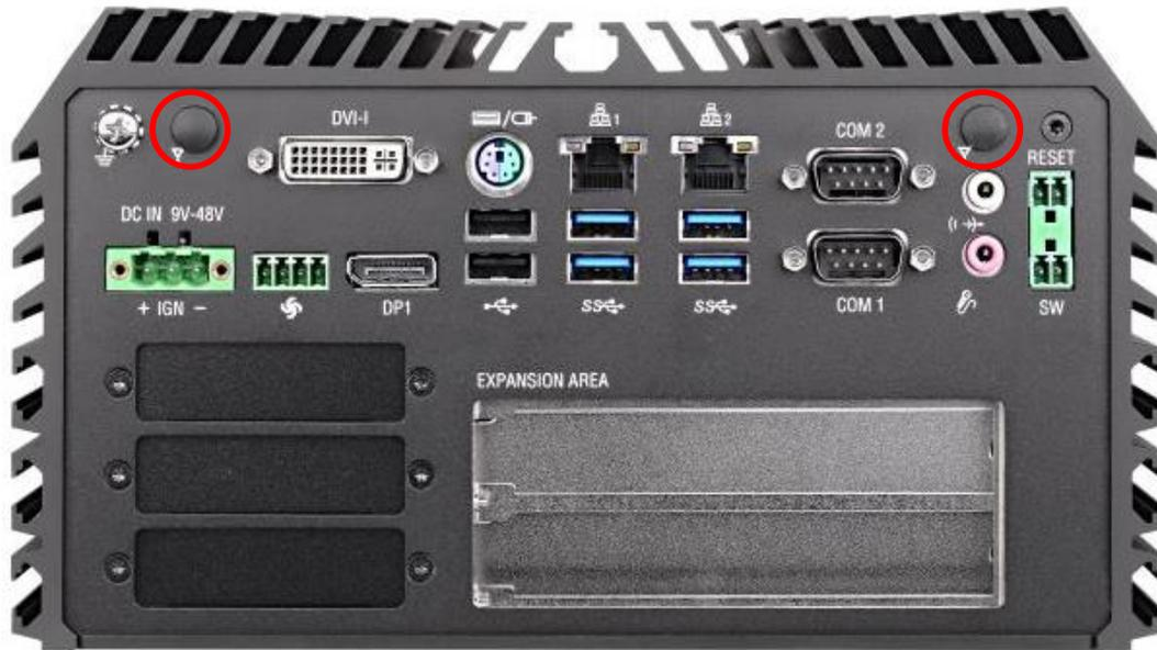
4. Loosen the 4 screws. Pull out 4 latches as marked on photo.
