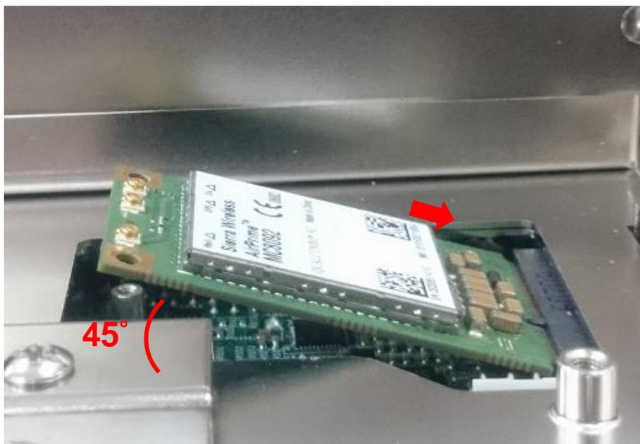
3. Press down the module and use previous two screws to fix the module.
