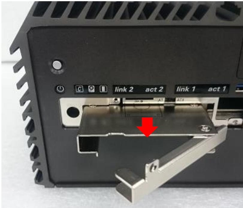
4. Make the PCB side of the HDD face up, place the HDD bracket into it. Ensure the direction of bracket is correct and use 4 provided screws to assemble HDD and HDD bracket together.
