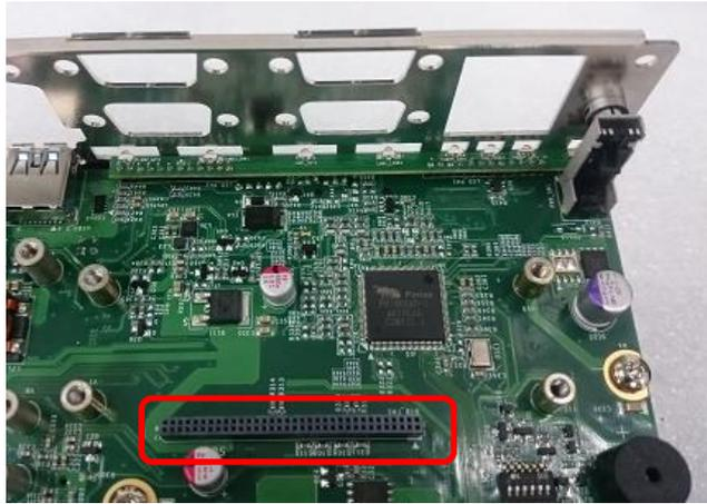
3. Insert the CMI module carefully into the CMI connector on main board.
