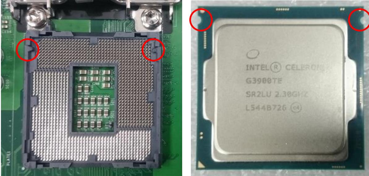
4. The notches of socket provide the space for fingers while lowering the CPU, hold the CPU by the edges toward the notches and insert the CPU gently.
