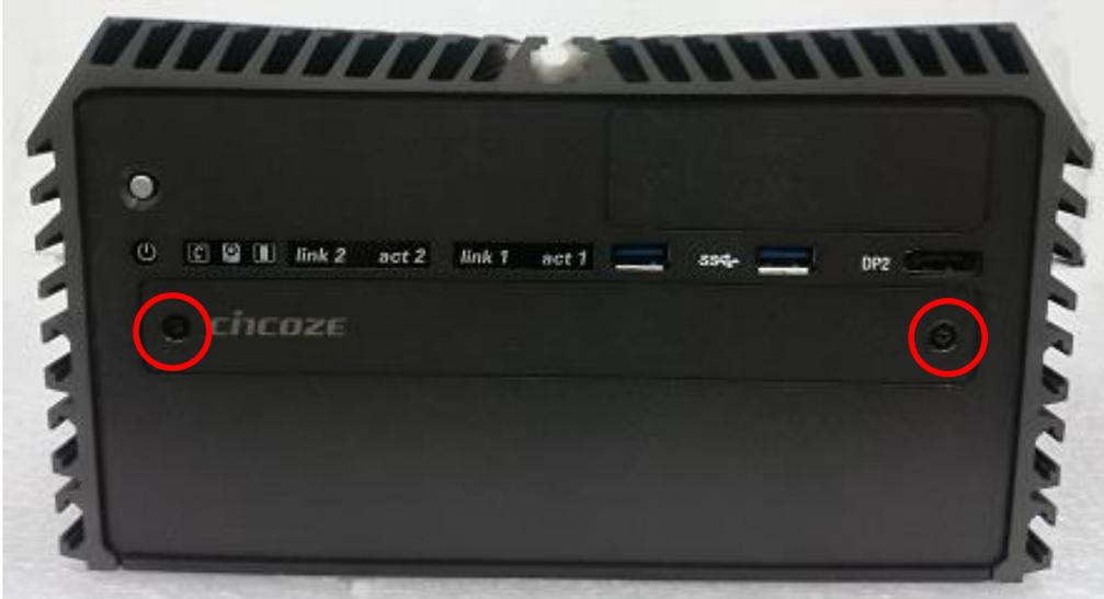
2. Locate the removable HDD bay and loosen the screw.
