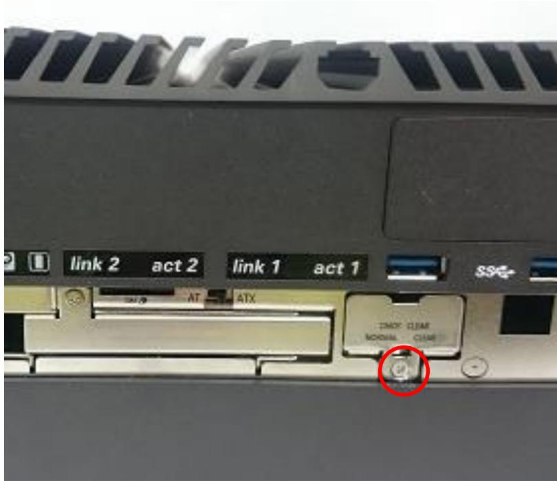
2. Pull out the CMOS battery bracket with assistance of a tweezer.
