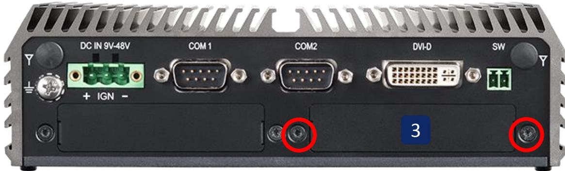
2. Attach the CMI-HD bracket on the backside of system's rear panel, and fasten it with two screws.
