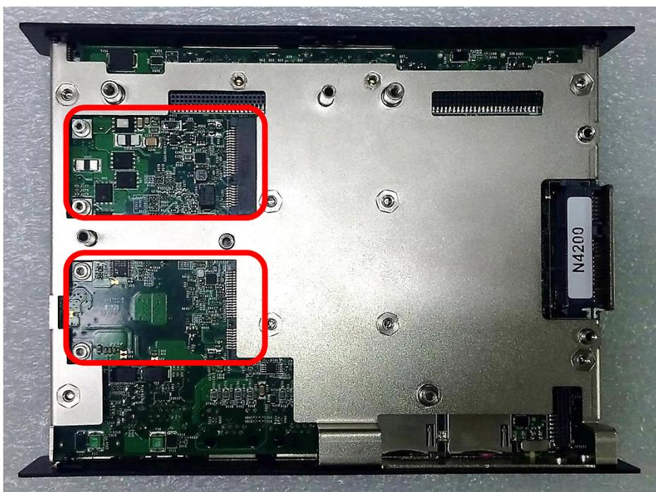
3. Tilt the Mini PCIe modules at 45 degrees angle and insert it to the slot until the gold-pated connector of module contacted firmly with the slot.
