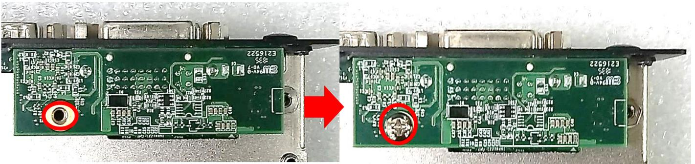
6. Attach the CMI-DVI bracket, and fasten 2 screws as marked.
