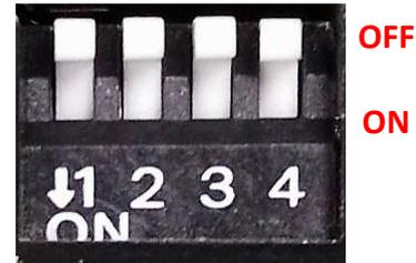
Default setting of Pin1 to Pin4 is OFF/ON/ON/ON.
