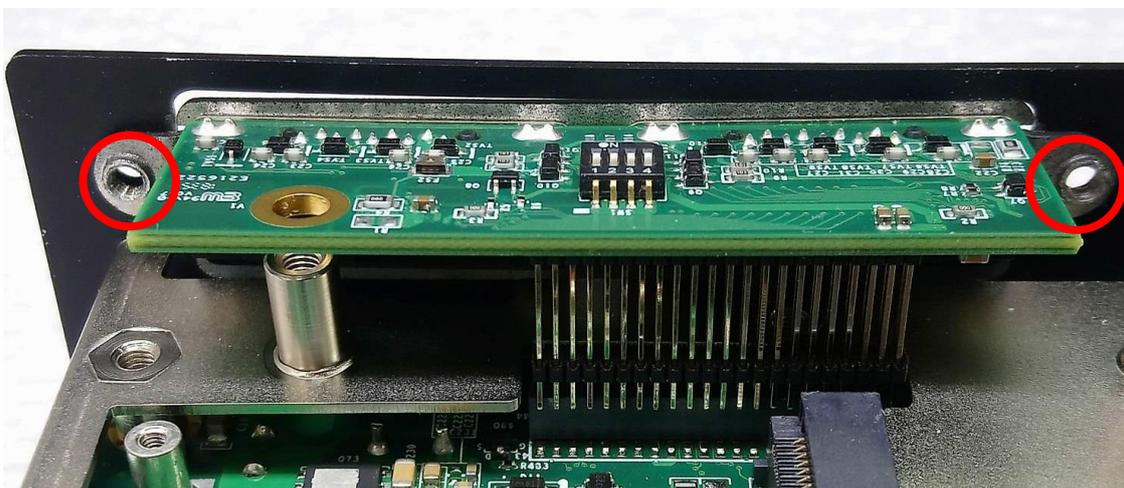
4. Push the connector pins on CMI-COM module until the pins can be inserted completely to the female connector (BTB\_FH2 or BTB\_FH1) on the system's mainboard.
