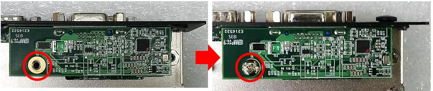
6. Attach the CMI-DVI bracket, and fasten 2 screws as marked.
