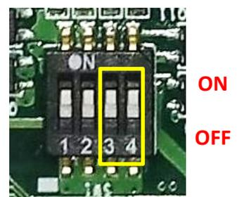
**SW1 on CMI-COM Module: COM5~6 with Power Select Switch****Function Setting via DIP Switch**
