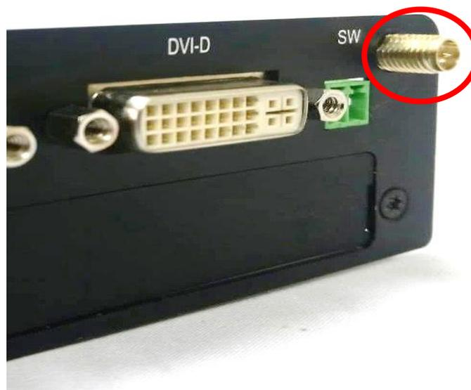
3. Put on washer and fasten the nut with antenna jack.
