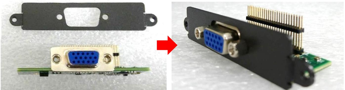
3. Align two holes on the CMI-VGA bracket with the holes on the rear panel.
