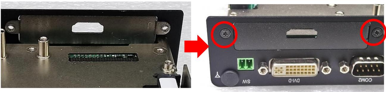
3. Align the hole on CMI-HD module with the screw hole on the system's mainboard module, and insert vertically to the female connector (BTB\_FH1) on the system's mainboard.
