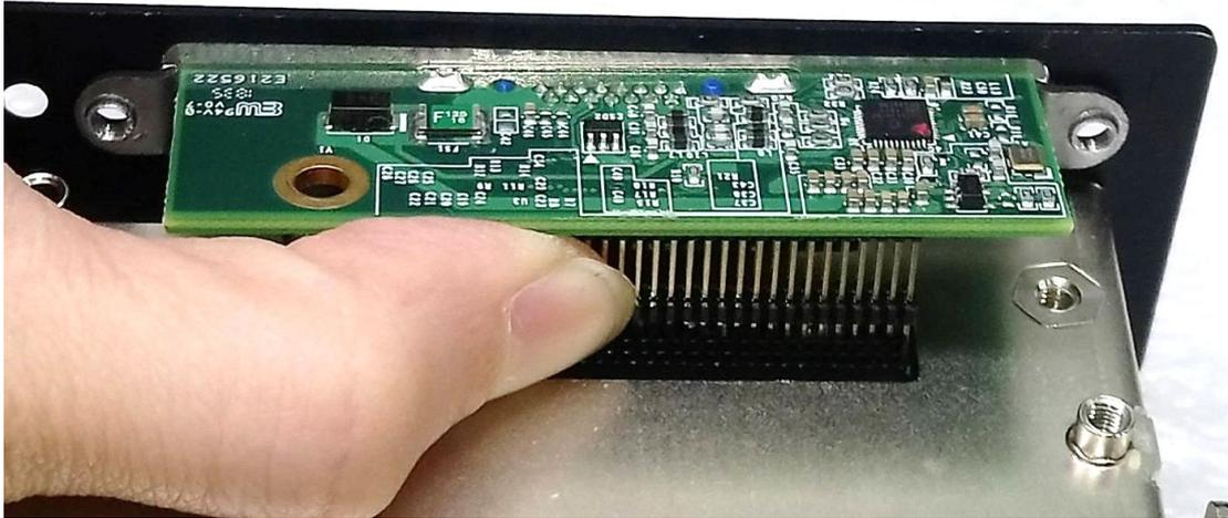
5. Make sure the hole on CMI-VGA module is aligned with the screw hole on the system's mainboard, and fasten a screw to fix it.
