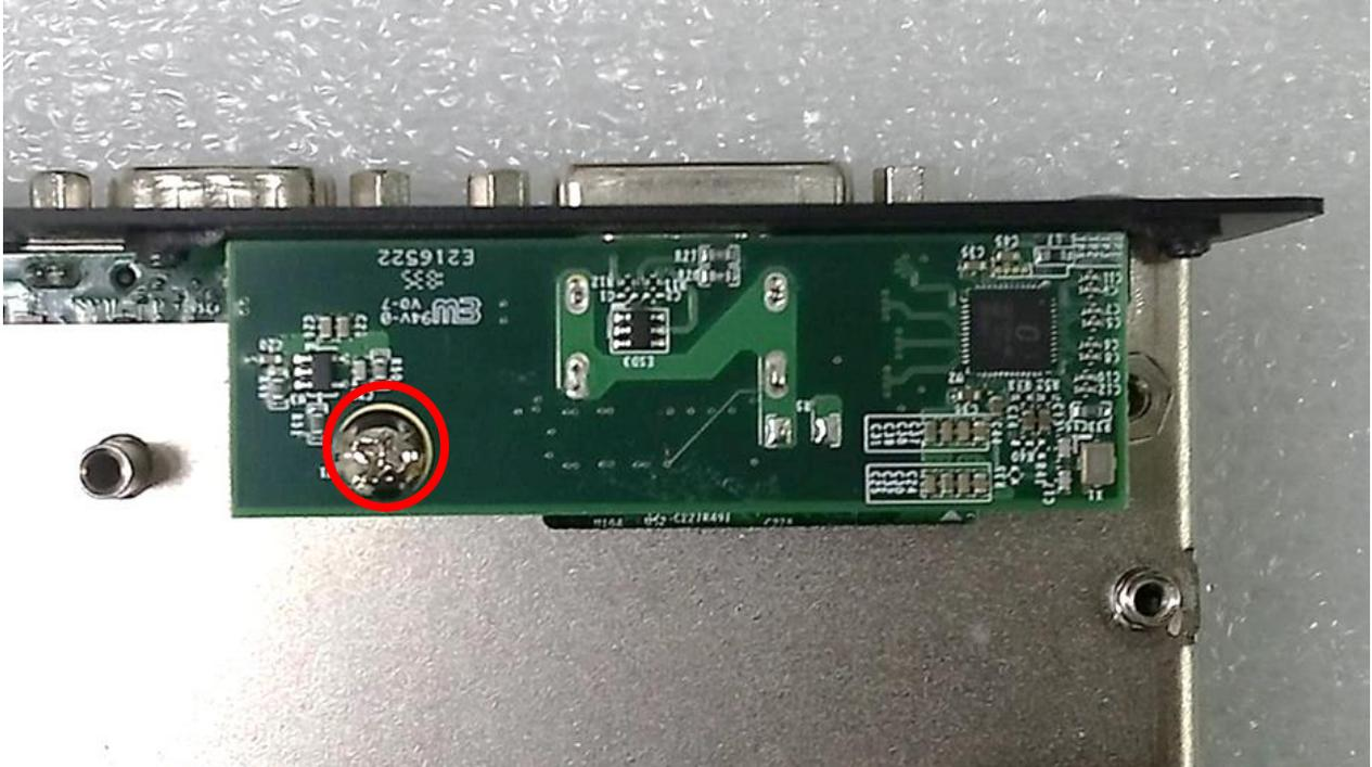
5. Align the hole on CMI-HD module with the screw hole on the system's mainboard module, and insert vertically to the female connector (BTB\_FH1) on the system's mainboard.
