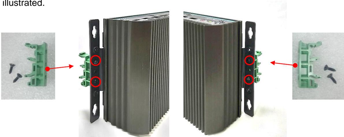
3. Clip the system into DIN rail as illustrated by the following steps. (1) Have lower end of mounting clip snaps into the DIN rail. (2) Press the system toward to have upper end of mounting clip snaps into the other side of DIN rail.
