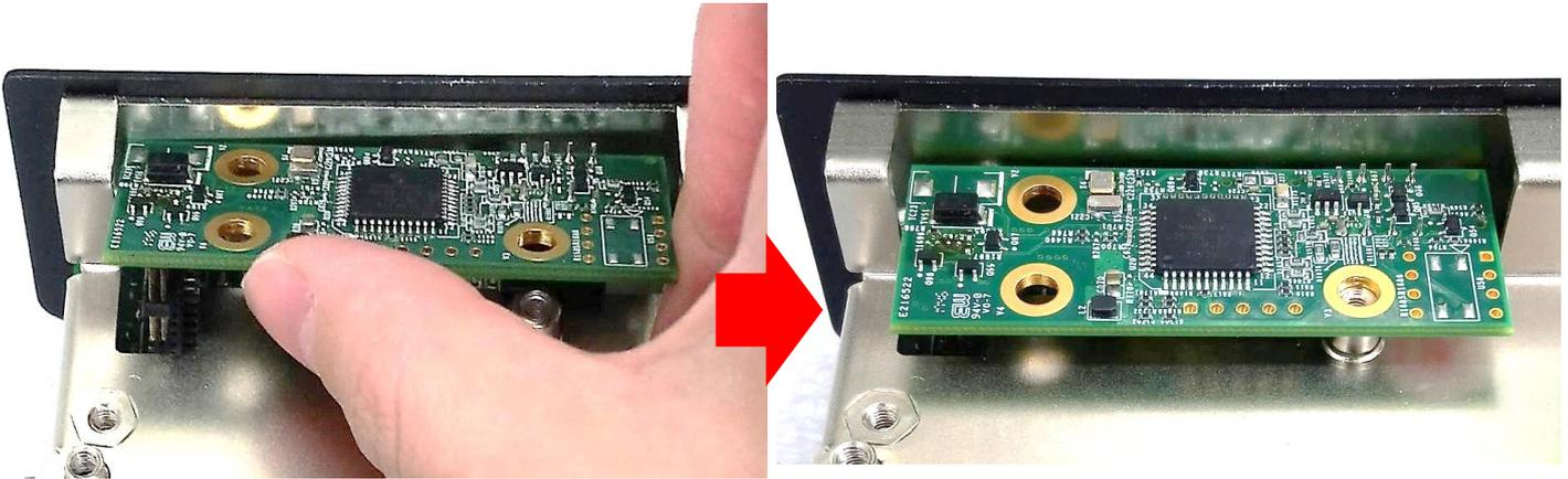
2. Fasten a screw to fix the CFM-IGN Module.
