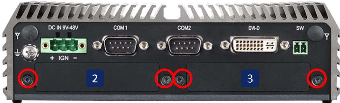
2. Assemble the CMI-COM bracket and CMI-COM module together with 4 D-Sub jack screws
