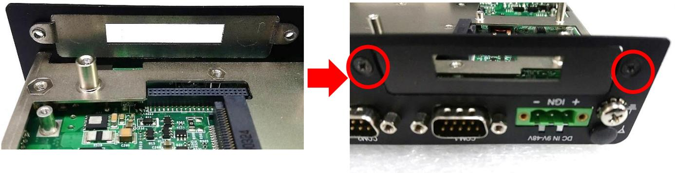
3. Push the connector pins on CMI-DIO module until the pins can be inserted completely to the female connector (BTB\_FH2 or BTB\_FH1) on the system's mainboard.
