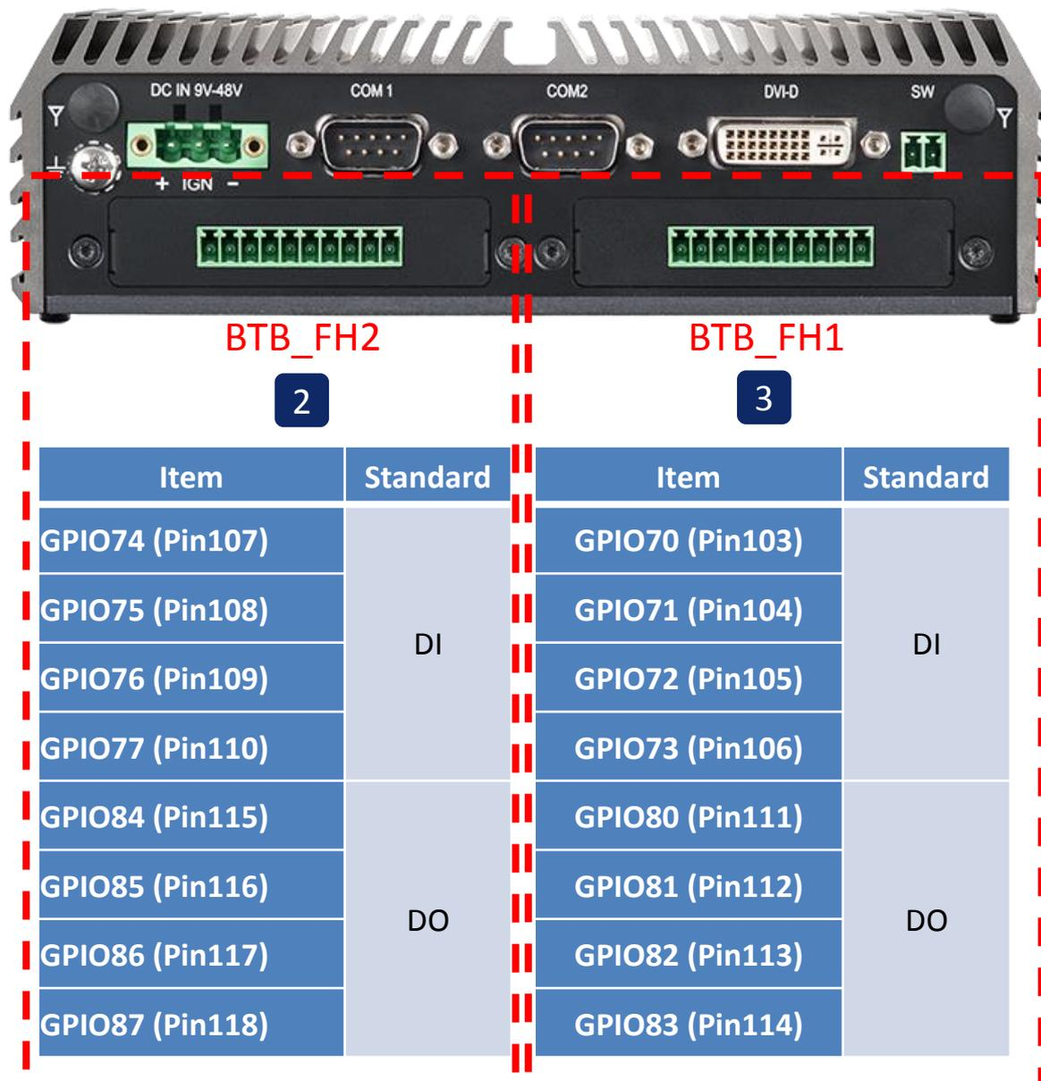
The image shows the rear panel of the DC-1200 fanless computer. A red dashed line highlights the BTB\_FH2 and BTB\_FH1 headers. Below the headers are two tables listing GPIO pins and their standards.
