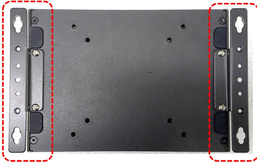
2. Fasten 2 DIN rail mounting clips to mounting brackets on both sides with provided 4 screws as illustrated.
