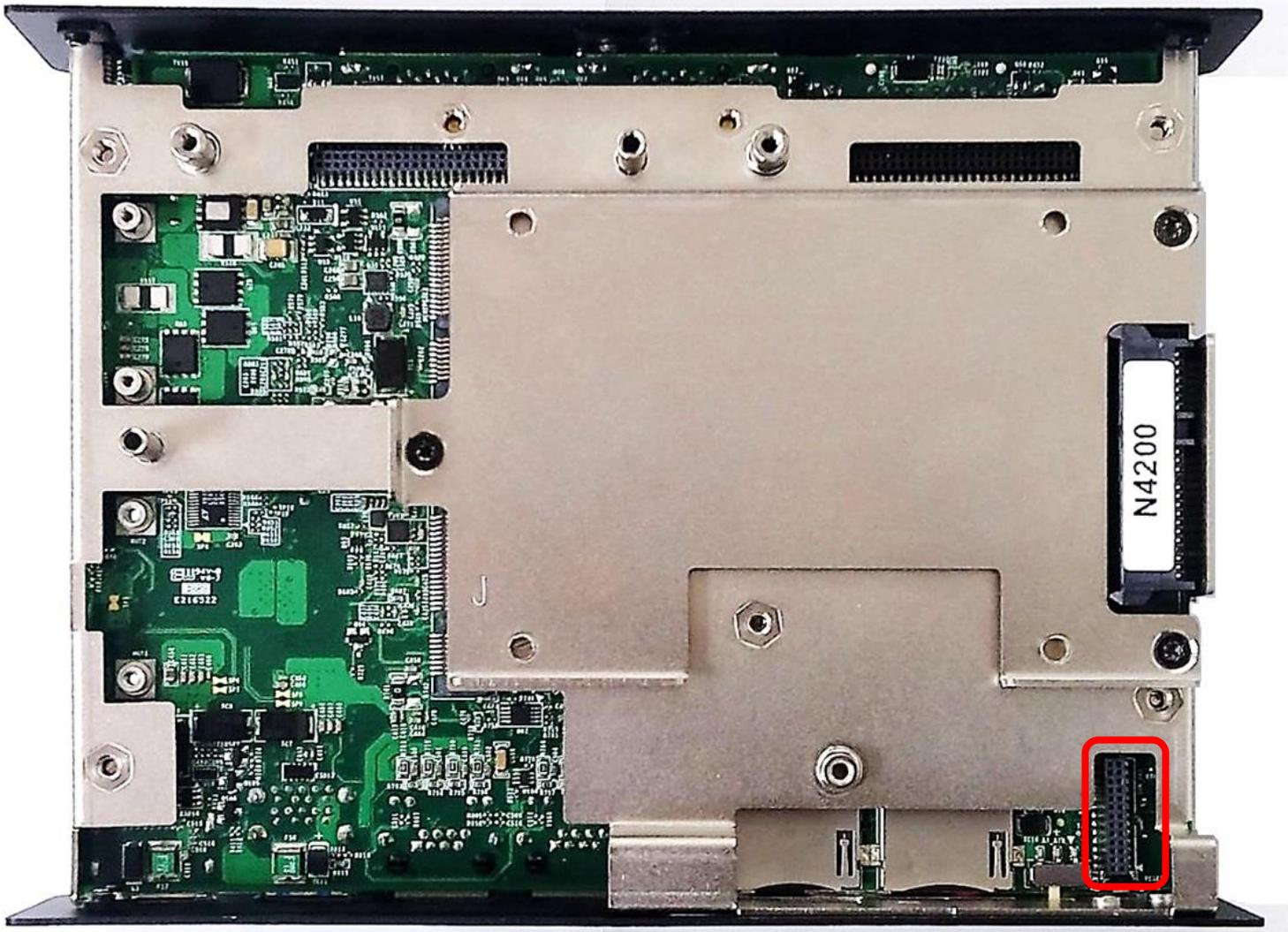
Locate the CFM-IGN Module's connector on system motherboard as indicated.
