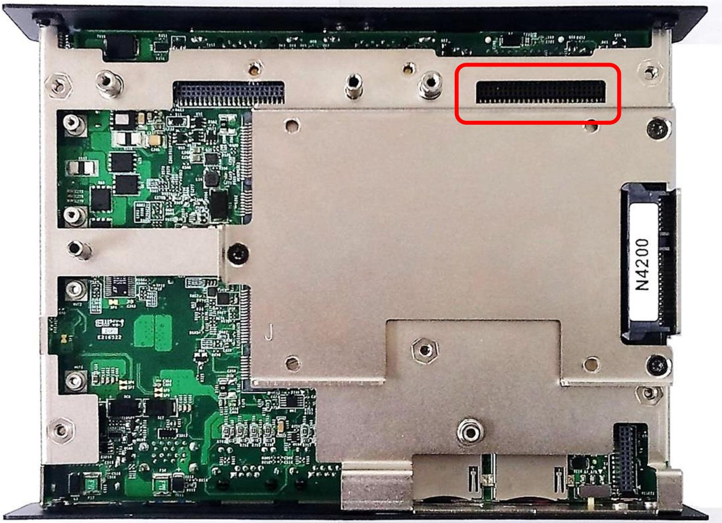
Locate the CMI Modules/ connectors on system motherboard as indicated.
