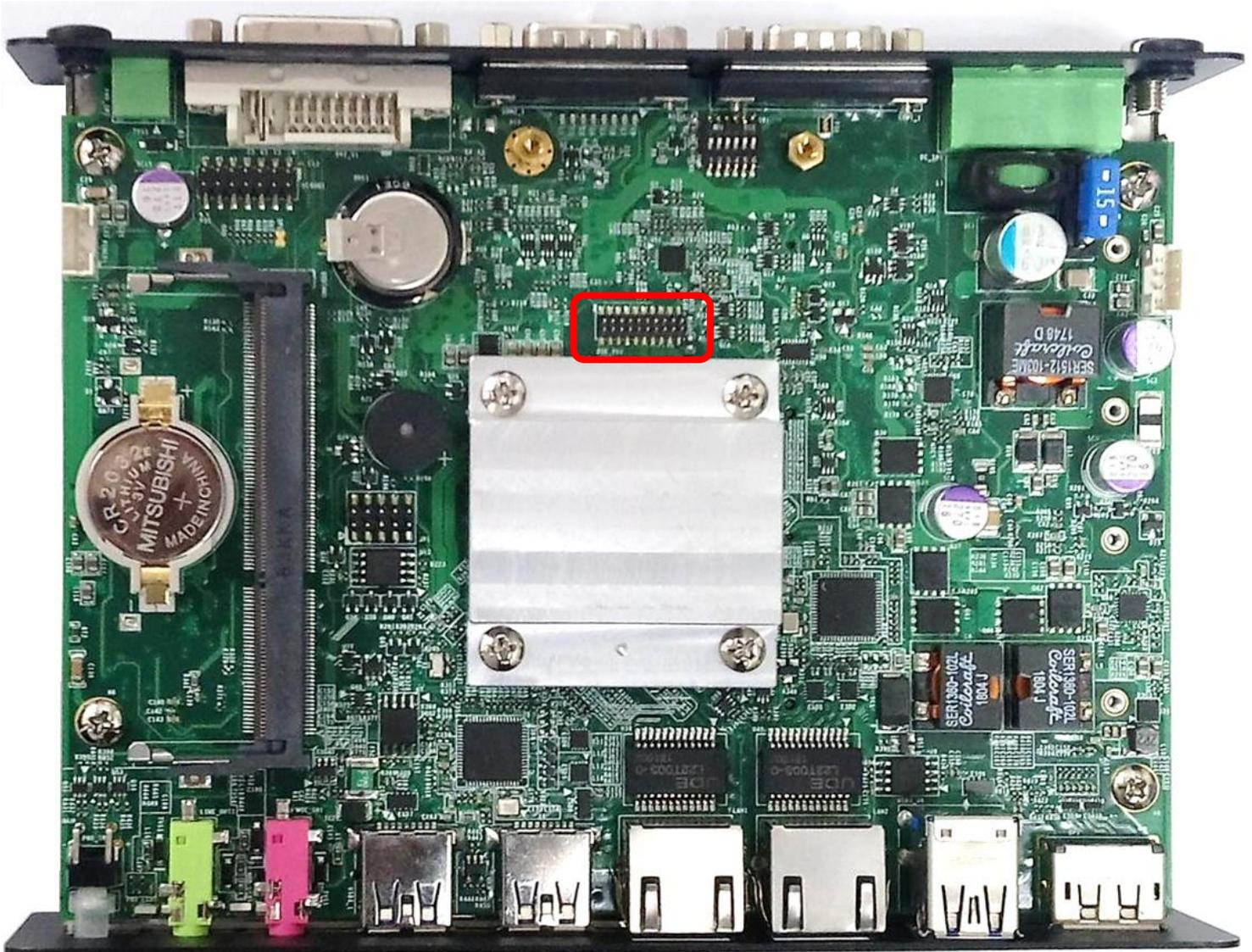
Locate the CFM-PoE Module's connector on system motherboard as indicated.
