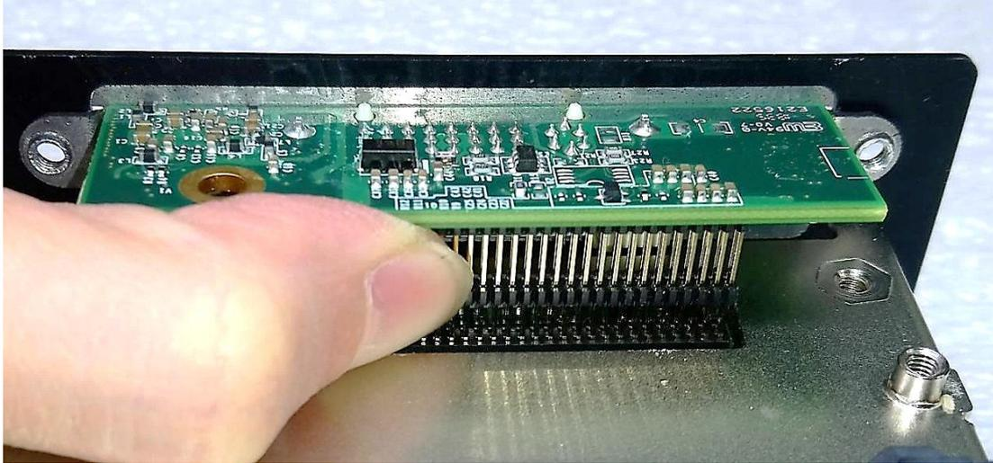
5. Make sure the hole on CMI-DVI module is aligned with the screw hole on the system's mainboard, and fasten a screw to fix it.
