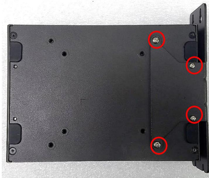
4. It is achievable to mount system on the wall by fastening the screws through the bracket mounting hole.
