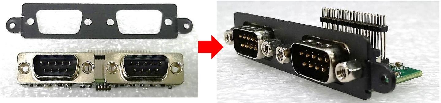
3. Align two holes on the CMI-COM bracket with the holes on the rear panel.
