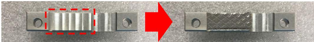
3. Paste the heatsink onto the CFM-PoE module carefully and fasten 2 screws to fix it.
