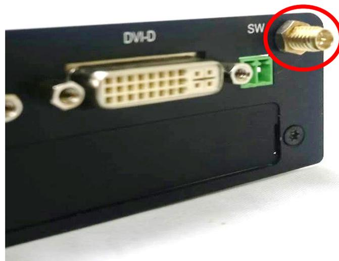
4. Assemble the antenna and antenna jack together.
