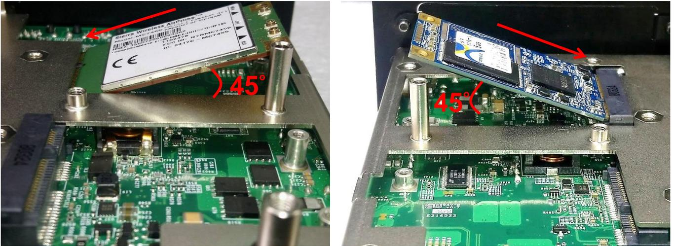
4. Press down the module and use two screws to fix a module.
