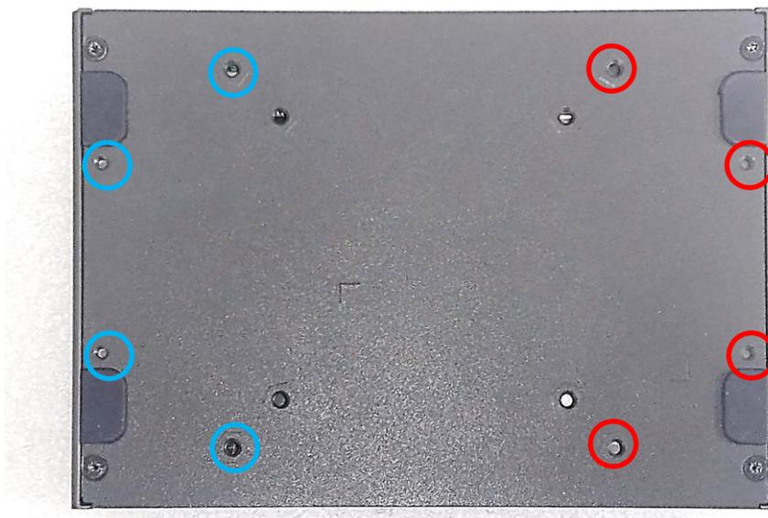
3. Place the side mount bracket on the bottom of system as shown in the picture below, and fasten the rest of 4 screws to fix the side mount bracket with system together.
