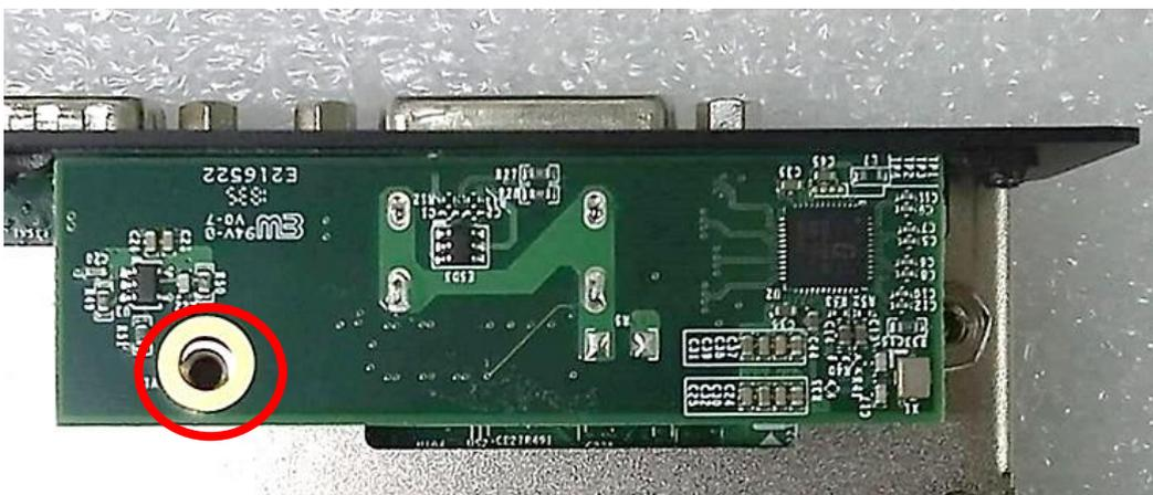
4. Fasten a screw to fix the CMI-HD module.
